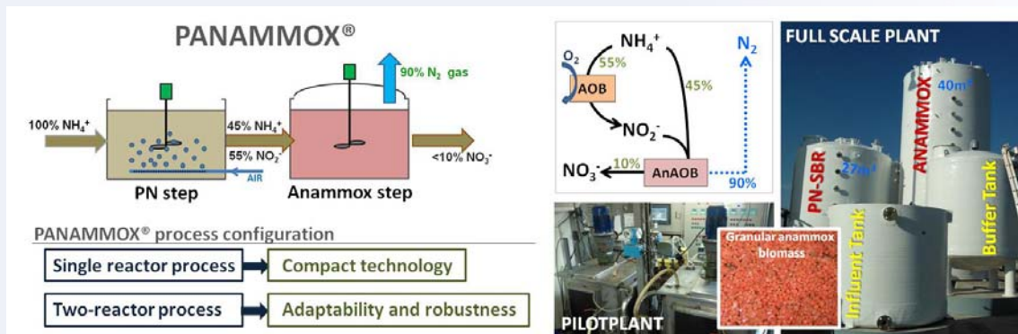
Overview of the PANAMMOX technology: scheme of the process and leachate treatment plants
